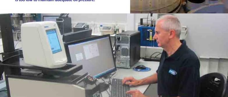
The Brookfield Viscometer measures the low temperature viscosity of gear oils and automatic transmission fluids. The test can be run at different temperatures depending on the grade, for example SAE 75W grades are tested at -40°C whereas SAE 80W oils are tested at -26°C.
